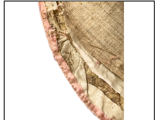
Original adhesive stabilizer, degraded and flaking.
